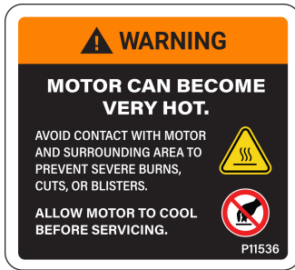
Figure 15: Warning - Motor Can Become Very Hot
