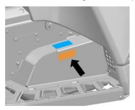
3. Apply the provided label P11531 "LABEL, ROTOR GUARD " to the designated area (ORANGE). (Blue indicates the existing label location).
