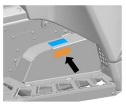
3. Apply the provided label P13198 "LABEL, ROTOR GUARD FR" to the designated area (ORANGE). (Blue indicates the existing label location).
