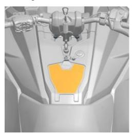
2. Apply the provided label P11526 "LABEL, PULLEY GUARD" to the designated area (ORANGE). (Blue indicates the existing label location).
